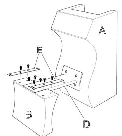
Use eight long bolts to attach the front base and the seat bracket bars.
